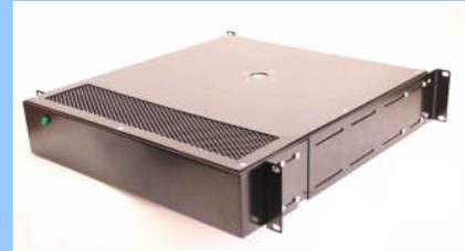
With the top perforated area of the fan tray protruding through the front 19-inch mounting angles the unit feeds air into a chimney created by a solid door, side panels, vertical baffles and equipment mounted in the cabinet. Any unused 19-inch apertures need to be blanked off to maximise cooling efficiency.
